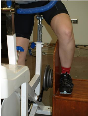
The safety foot platform device displayed allowed participants to place their non-exercising lower limb on the platform next to the stationary ergometer. Thus, the platform also acted as a shield protecting the participant from the rotating counterweight.
