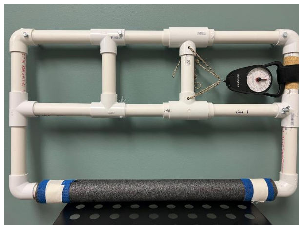
Figure 1: Device for participants to perform the palm press MVIC for the pectoralis major clavicular
